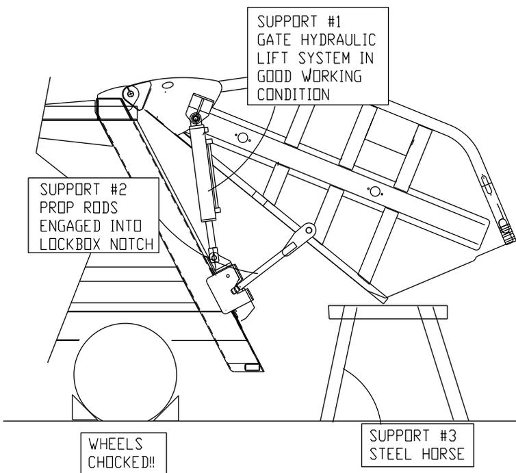
8- Once you are *completely satisfied* that the partially raised tailgate is secured in three ways in this raised position, institute your shop's detailed LOCKOUT/TAGOUT procedure.
