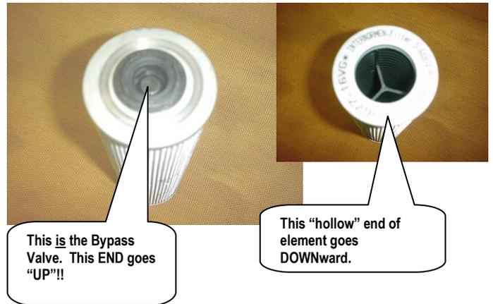
6- Now re-install the filter housings COVER. Snug up with MEDIUM force.
