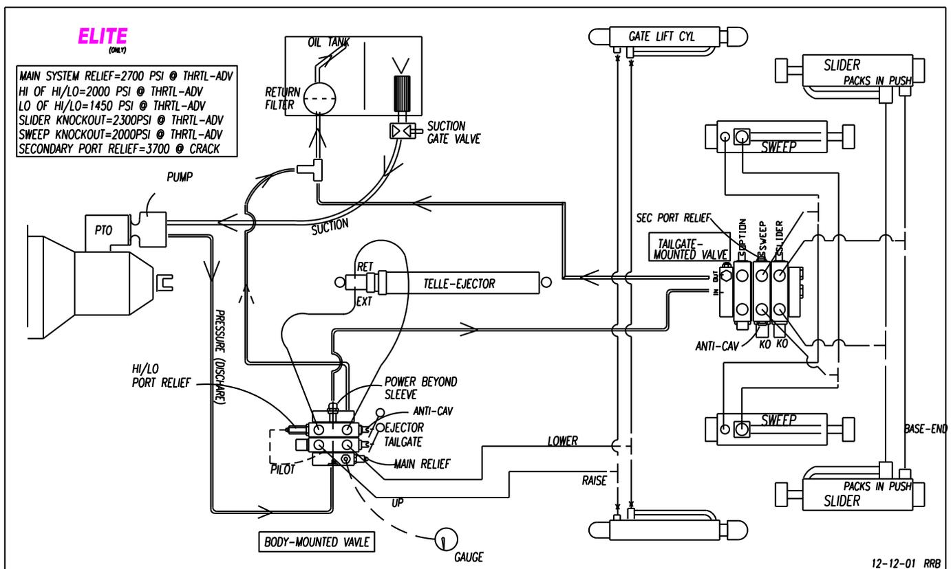
The position of the tailgate itself determines the pressure in pilot hose since the pilot hose connects to the tailgate *raise* plumbing. If the tailgate is raised (at time of payload pushout), the weight of the tailgate "induces" a pressure much greater than the 750 PSI threshold and the hi/lo shifts to its high setting and the full 2000 PSI @ throttle advanced is available for "pushout".
