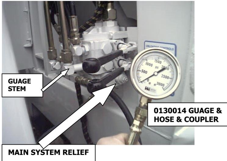
To check the setting of the system "main relief", do the following procedure.
