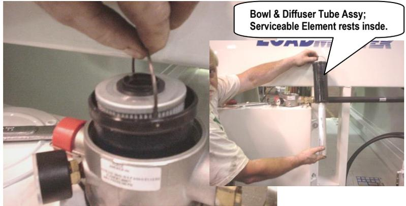
4- Now remove the "old" element. Put it into clean garbage bag so you can later "study" what has been trapped-out of the hydraulic system (can offer "clues" as to the hydraulic system's "health").
