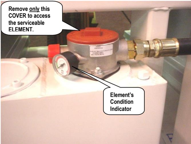
2- Remove the Filter's Top Cover by turning CCW. The Cover's compression spring will be "pushing"...so use your hand over the Red removable polymer cover when it is close to being fully un-threaded to control.
