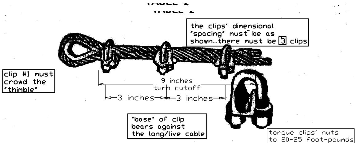
**NOTE: There is only one correct method of installing wire rope clips. They should be attached to rope ends as shown in photograph above. The base of each clip should bear against the live, or long rope end, and the U-Bolt should bear against the dead or short rope end.**
