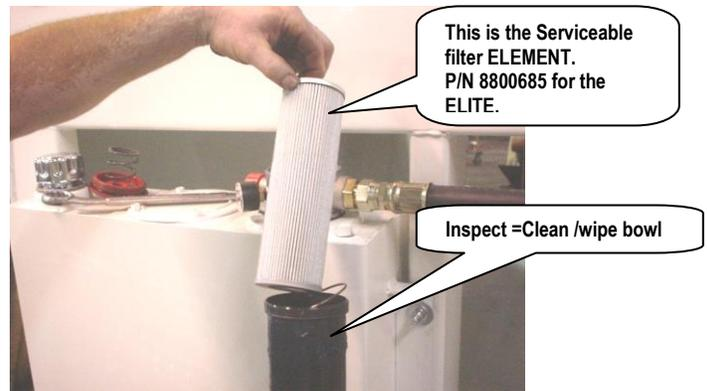
5- Insert fresh element into the Bowl...this element has a "built-in" Bypass Valve. Assure the Bypass Valve is "UPWARD".
