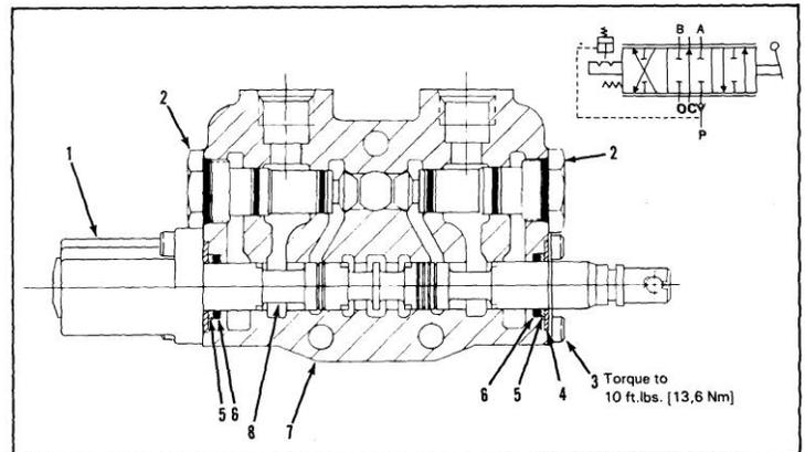
Figure 4-5. 4-Way, 3-Position Valve Section with Pressure Detent Release.
