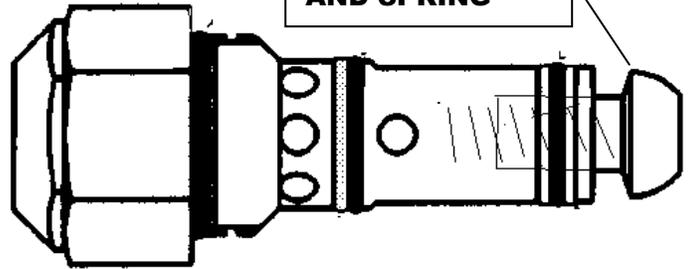
A typical "symptom" that might lead you to replace this cartridge is that the sweep blade is "tending to unwrap" when the body is nearing its full rated payload capacity. Be careful in your observations here because some occasional unwrap of sweep blade is *normal* (such as when the body is *NEARLY full* and the payload is at its rated value).
